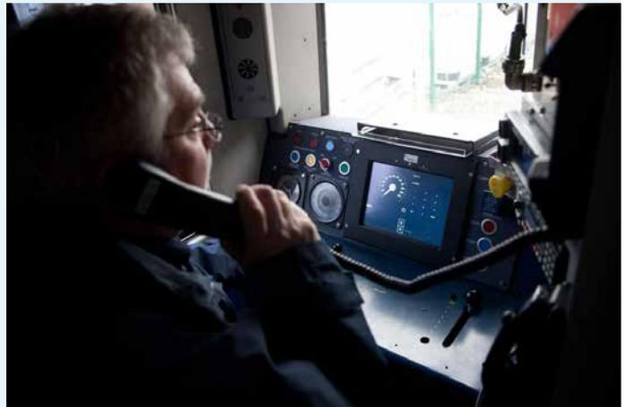
The driver of a Class 158 on the Cambrian with the ERTMS screen (Driver Machine Interface) showing target speed.
